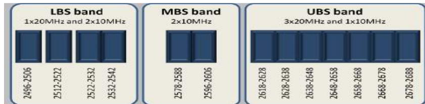
FDD-LTE with 20MHz channels overlaid on WiMAX
